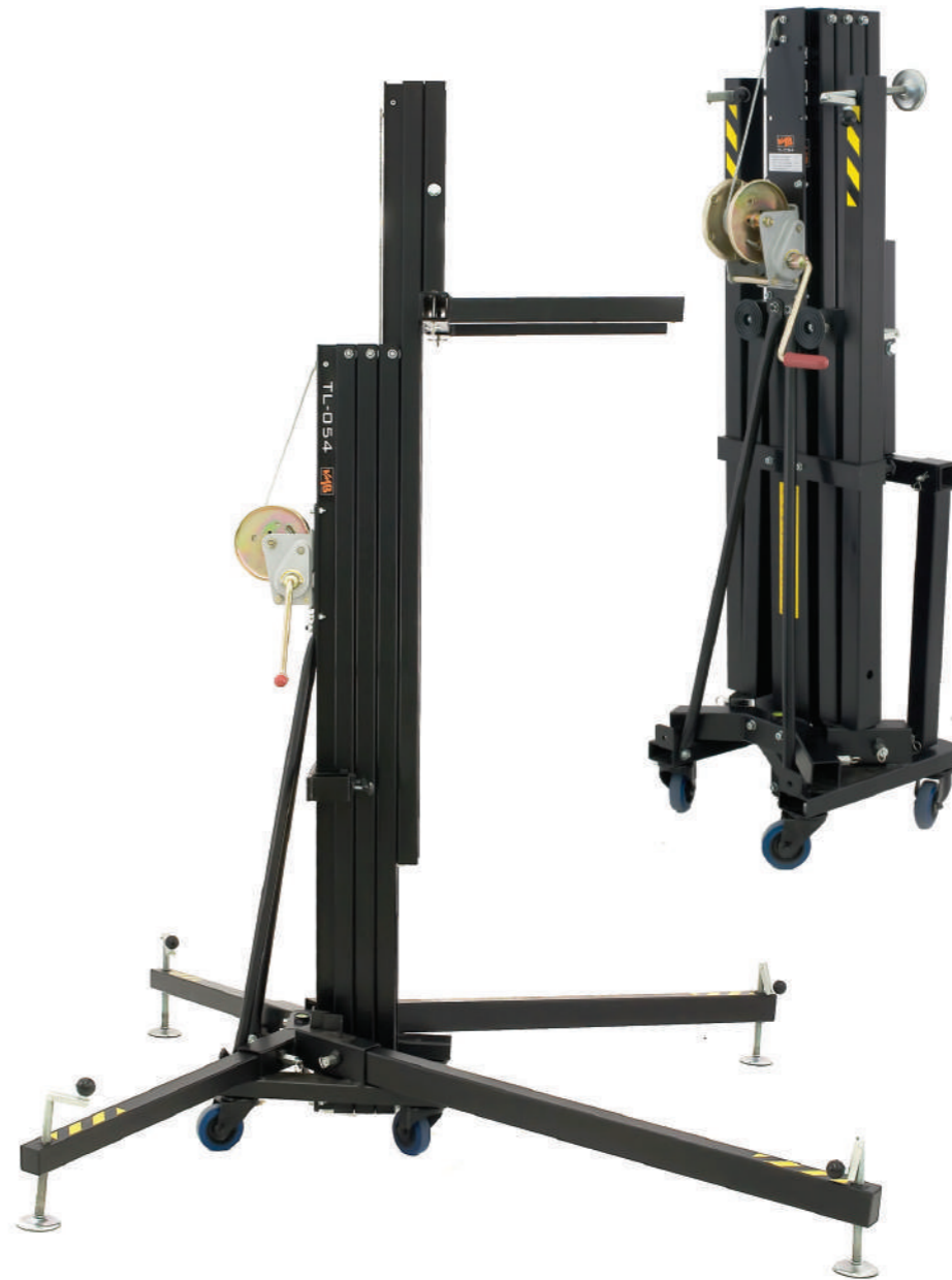
The profiles automatically rise in sequence thanks to the SRS (Sequence Retainer System).
